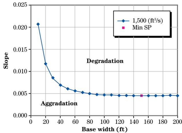
**Figure 9-21** Stability curve depth versus base width,  $Q = 1,500 \text{ ft}^3/\text{s}$ , bed-material sediment concentration = 1,917 mg/L. Limerinos resistance and Meyer-Peter and Müller sediment transport equations
