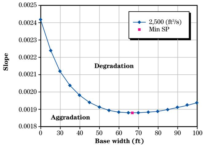
**Figure 9-18** Stability curve depth versus base width,  $Q = 2,500 \text{ ft}^3/\text{s}$ , bed-material sediment concentration = 211 mg/L. Brownlie resistance and sediment transport equations
