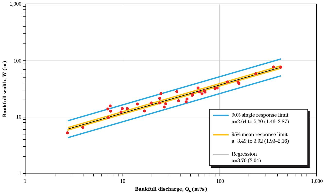
**Figure 9-12** Downstream width hydraulic geometry for U.K. gravel-bed rivers,  $W = aQ_b^{0.5}$  with confidence bands. Based on 43 sites in the U.K. with resistant banks. SI units m and  $m^3/s$  (English units ft and  $ft^3/s$ )
