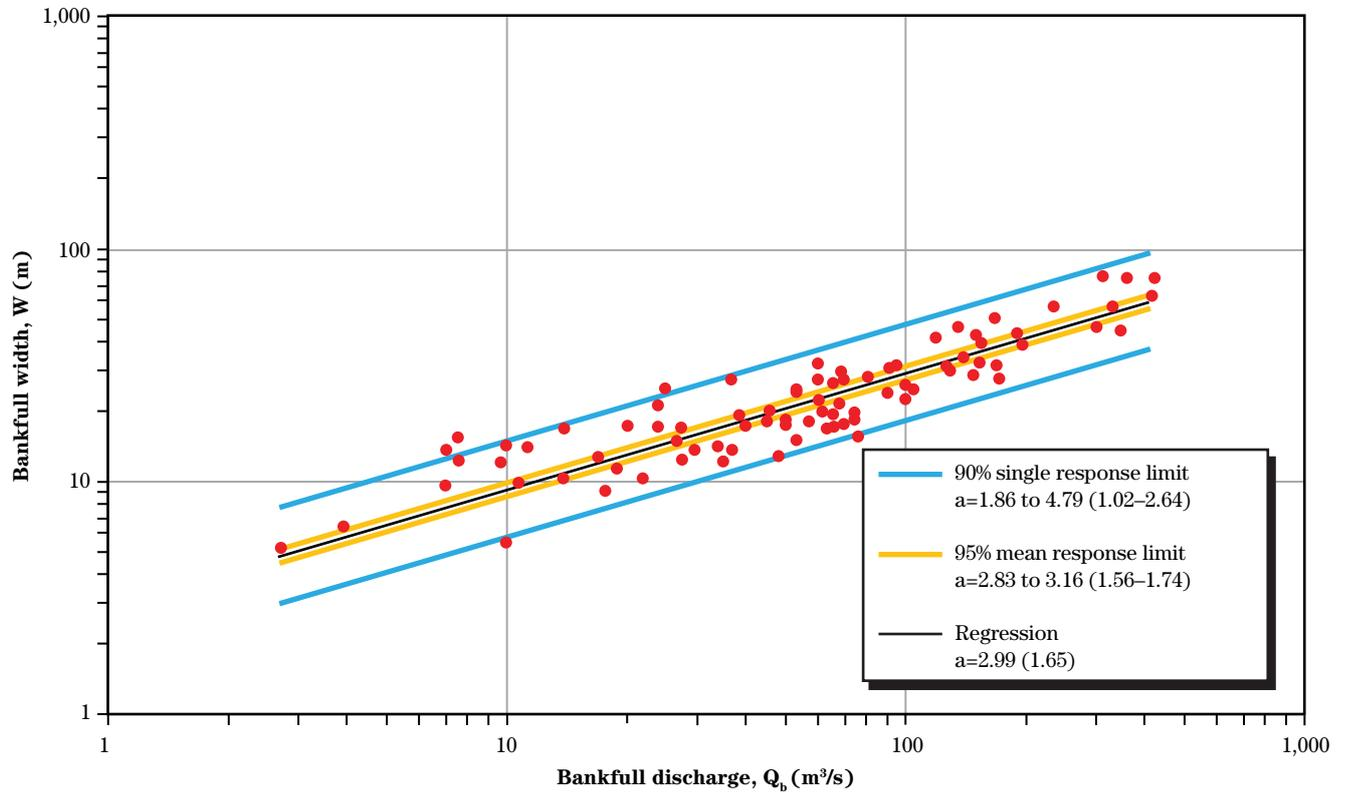
**Figure 9-11** Downstream width hydraulic geometry for U.K. gravel-bed rivers,  $W = aQ_b^{0.5}$  with confidence bands. Based on 36 sites in the U.K. with erodible banks. SI units m and  $m^3/s$  (English units ft and  $ft^3/s$ )
