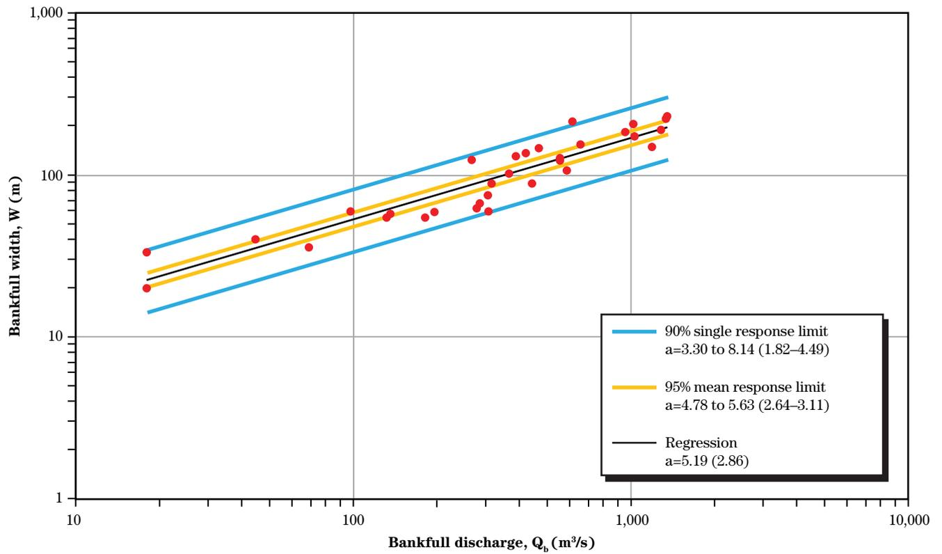
**Figure 9-5** Confidence intervals applied to the width hydraulic geometry equation based on 26 sand-bed rivers with at least 50% tree cover on the banks (T2). SI units – m and m<sup>3</sup>/s (English units ft and ft<sup>3</sup>/s)
