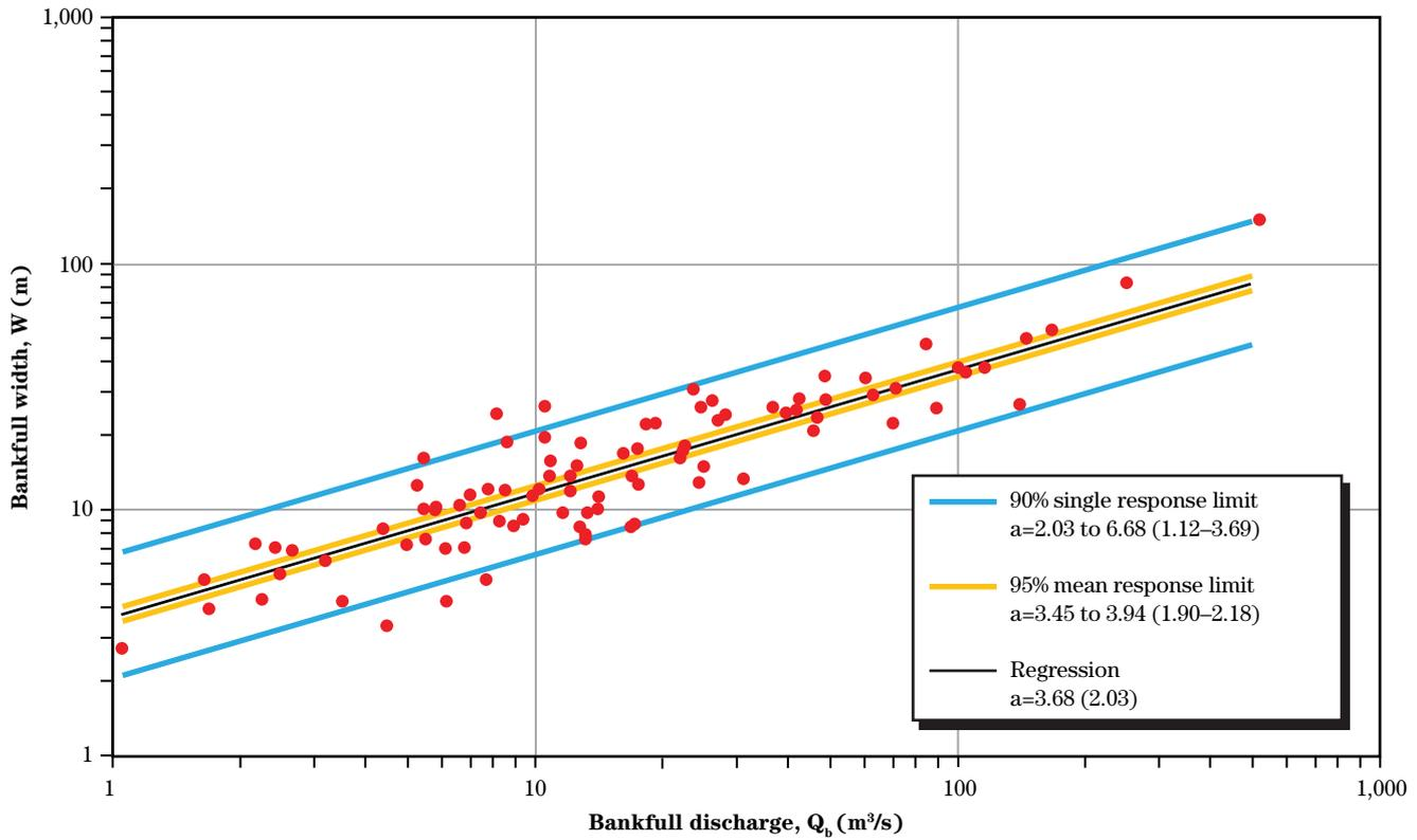
**Figure 9-10** Downstream width hydraulic geometry for U.K. gravel-bed rivers,  $W = aQ_b^{0.5}$  with confidence bands. Based on 86 sites in the U.K. SI units m and  $m^3/s$  (English units ft and  $ft^3/s$ )
