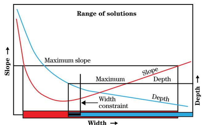
**Figure 9-15** Stability curves for channel-forming (stable channel) discharge and a flood discharge
