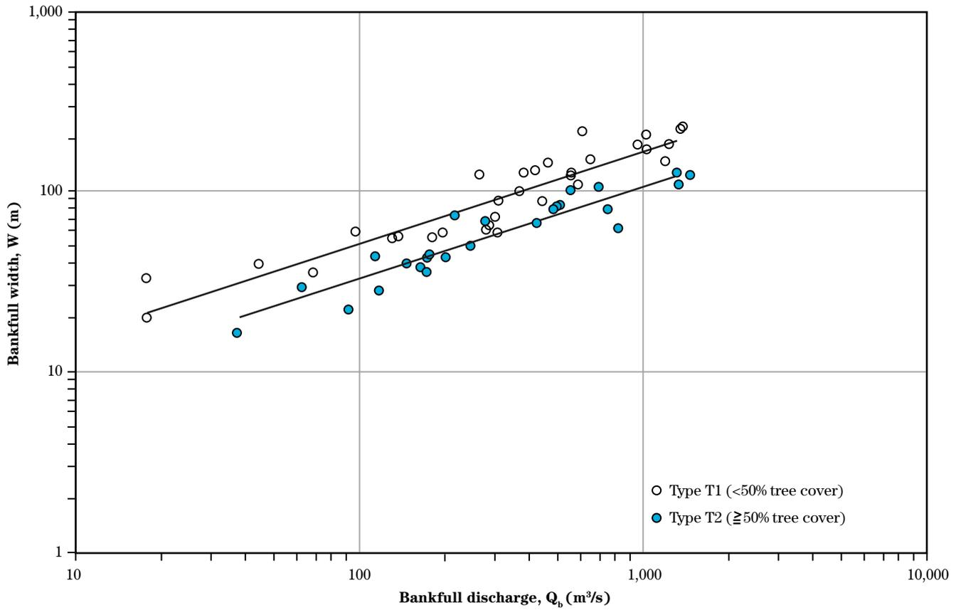
**Figure 9-3** Sites used to develop U.S. sand-bed river hydraulic geometry relationships
